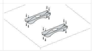
3. Secure the fan on the bracket with clamps and bolts removed earlier. Suspend the fan carefully. Make sure the fan is fastened securely prior to operation.
