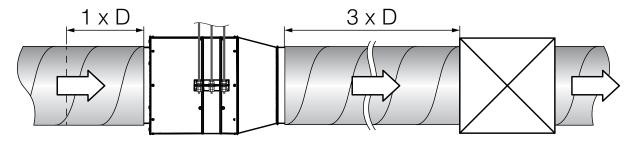
To attain the best performance of the fan and to minimise turbulence-induced air pressure losses connect the straight air duct section to the spigots on both sides of the unit while mounting.
