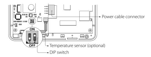
Temperature sensor — room temperature sensor. If physically present in the panel configuration, select "Sensors in control panel" item in the control panel menu.
