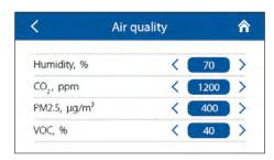
Set threshold values for the humidity,  $CO_2$ , PM2.5, and VOC sensors. The unit will automatically maintain the user values by smoothly increasing or decreasing the fan speed.
