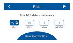
Setting the filter maintenance timer: upon elapsing of a pre-set period of time (70–365 days) the main page will show a filter replacement alert while the **Alarms** window will display the respective information about the necessary filter change. To disable the filter timer (e.g. if the unit is equipped with pressure switches), set the value to 0 days.
