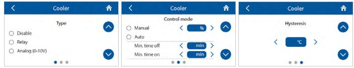
Select the cooler type (discrete/analogue) and its operation mode.
