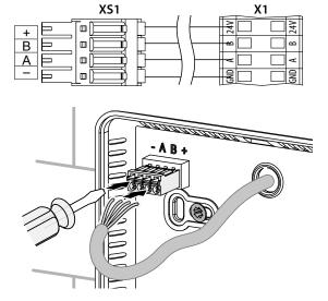
**5.** Remove the connector with the cable from the bracket and connect it to the female connector on the circuit board.
