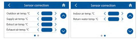
The sensor readings are corrected by entering values with horizontal arrow keys in the range from -50.0 °C to +50.0 °C.
