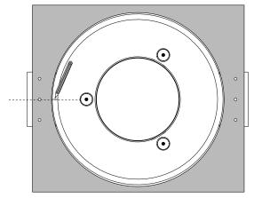
For comfortable mounting, locate the mounting template on the internal packing attachment. Align the template with the diffuser and make a mark coaxial to the hole in the middle.
