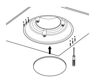
Secure the diffuser with screws. Install the front panel fixed with magnet holders.
