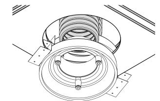
Install the air duct onto the diffuser's flange.
