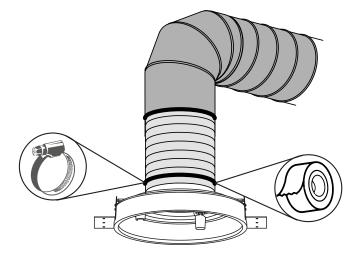
Secure the connection with the worm drive clamp or duct tape.
