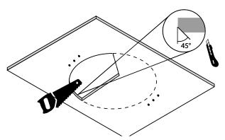
Align the template with the ceiling and mark up the places to install the diffuser and make holes for mounting. Make a hole in the drywall. Remove the chamfer at a 45° angle up to 1/3 drywall thickness.
