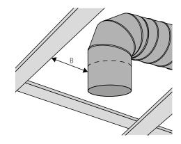
ATTENTION! To prevent vibration, a section of flexible duct must be attached in between the diffuser and rigid duct.
