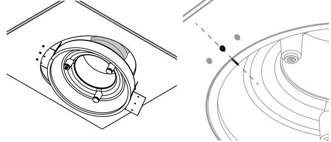
Install the diffuser into the hole in the ceiling. The mounting brackets must be supported with the back side of the drywall. Align the mark on the diffuser with the center of the hole in the middle.
