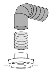
To attach the mounting brackets to drywall, use screws at least 3.9 mm in diameter.
