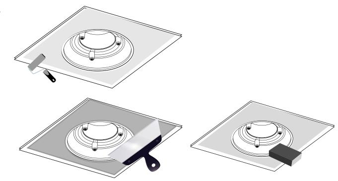
Apply the primer ("Knauf Tiefengrund" or similar). When dry, putty ("Knauf HP Finish" or similar) and grind on the surface.
