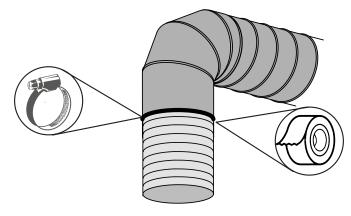
Connect the flexible air duct to rigid air duct. Fix the connection with the worm drive clampor duct tape.
