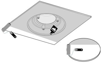
Apply the primer (the one recommended by the paint's manufacturer). Paint the diffuser and the drywall.
