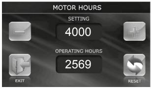
The **MOTOR HOURS** function enables the user to set up filter cleaning or replacement periodicity. Upon expiration of the preset time the panel displays a filter cleaning or replacement indicator. The indicator is displayed every 24 hours.
