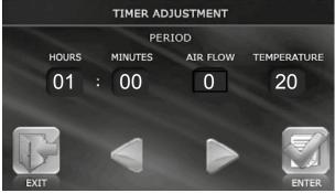
• To activate the timer, press **TIMER** in the control panel Main menu.
