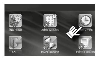
• To set the date and time on the control panel, go to the User menu by pressing (see para. 5) and then press **DATE, TIME**.
