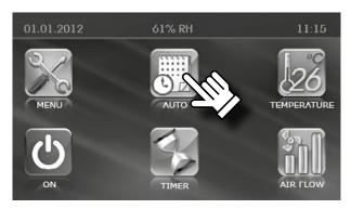
• The **AUTO** mode enables scheduled operation of the ventilation unit. The unit runs at the preset speed and temperature during the specified time periods.
