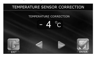
• To correct the panel temperature sensor indications, select **TEMPERATURE CORRECTION** submenu from the Engineering menu and press
