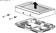
• Connect the cable to the control board and install the frontal part of the panel using the screws.
