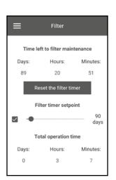
Filter timer setpoint: When the set time (70-365 days) has elapsed, the filter change indicator appears and filter replacement information is displayed in the Alarms menu. To disable the timer, remove the selection next to the slider of filter timer setpoint. If the unit is equipped with filter contamination control pressure switches, once the timer is disabled the filter contamination is signalled by the pressure switches only.
