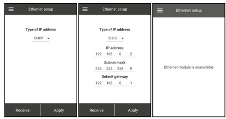
Press the **Receive** button to display the current Ethernet settings.
