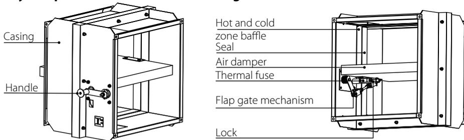
**The BSK2...PKP/BSK2...PVP/BSK2...PSP fire safety damper with a Belimo electric actuator and thermoelectric breaker**
