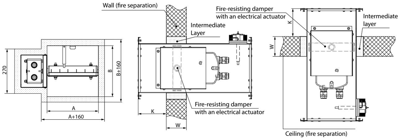
**INSTALLATION RECOMMENDATIONS FOR BSK2...72S DAMPERS WITH A THERMAL FUSE AND A RETURN SPRING**
