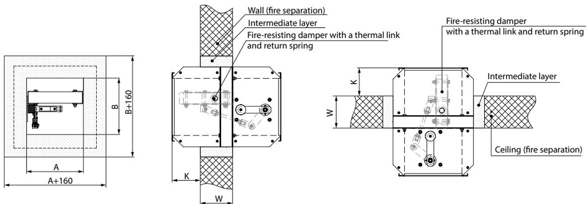
**INSTALLATION RECOMMENDATIONS FOR BSK2...PKP/BSK2...PVP/BSK2...PSP FIRE SAFETY DAMPERS WITH ELECTRIC ACTUATOR AND THERMOELECTRIC BREAKER**
