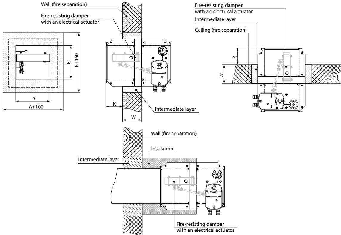
**INSTALLATION RECOMMENDATIONS FOR BSK2...PKP...S/BSK2...PVP...S/BSK2...PSP...S FIRE SAFETY DAMPERS WITH AN ELECTRIC ACTUATOR AND THERMOELECTRIC BREAKER**
