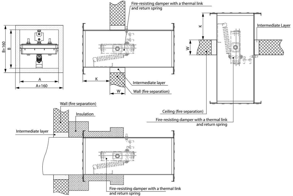
**INSTALLATION RECOMMENDATIONS FOR BSK1...PKP/BSK1...PVP/BSK1...PSP FIRE SAFETY DAMPERS WITH ELECTRIC ACTUATOR AND THERMOELECTRIC**
