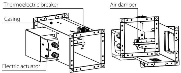
**The BSK2...72S fire safety damper with a mechanical actuating unit with a thermal fuse and a return spring**
