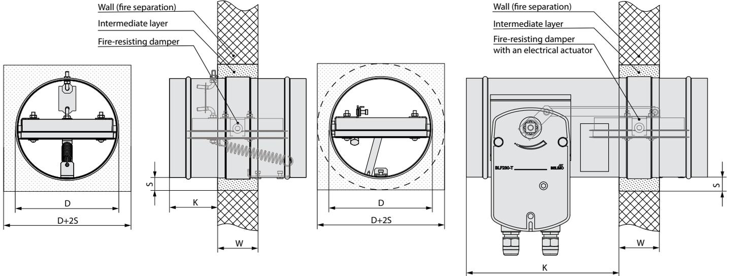
Fire-safety dampers can be installed into solid ceiling panels with the minimum thickness of  $W = 150$  mm, minimum intermediate layer thickness  $S = 50$  mm. The ceiling panels are made of concrete. The intermediate layer can be made of concrete or mortar. While carrying out the installation mind size  $K$ .
