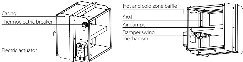
**The BSK2...PKP...-1/BSK2...PVP...-1/BSK2...PSP...S fire safety damper with a Belimo electric actuator and thermoelectric breaker**
