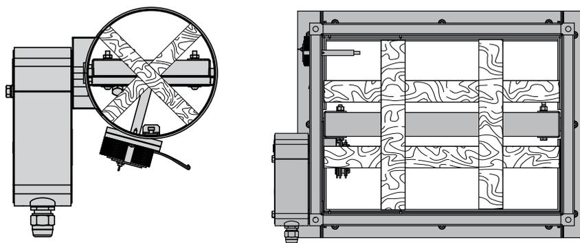
Following the damper installation into the shaft, wall or ceiling filler structure section and upon complete curing (immobilization) of the mortar make sure to remove the wooden spreader bars. The damper must open and close freely without excessive friction.
