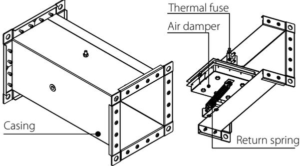
**BSK1...PKP/BSK1...PVP/BSK1...PSP fire safety damper with a Belimo electric actuator and a thermoelectric breaker**
