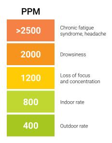
CO2 sensors can operate both as individual autonomous devices and in conjunction with ventilation equipment. In the latter case, the ventilation device can automatically turn on and off, as well as change its operating modes depending on the concentration of carbon dioxide in the room.
